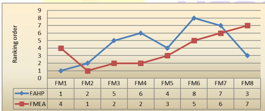
Figure (2): ranking comparison of priority in the traditional and proposed method
